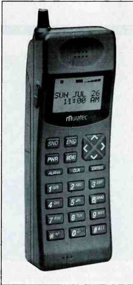
The Murata/Muratec CT-150 is a dual-mode analog/digital cellular that offers some clever features.
